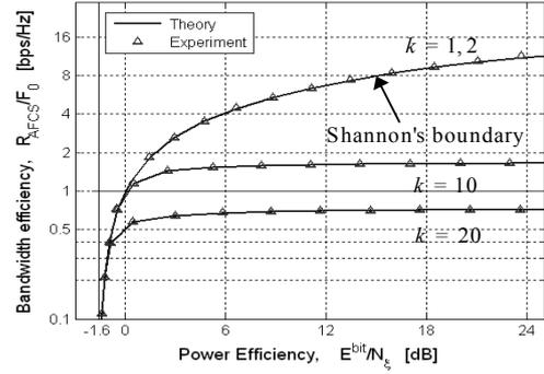
Fig. 3. Changes of power-bandwidth efficiency of optimal AFCS depending on the number of transmission cycles (results of computer experiment)
